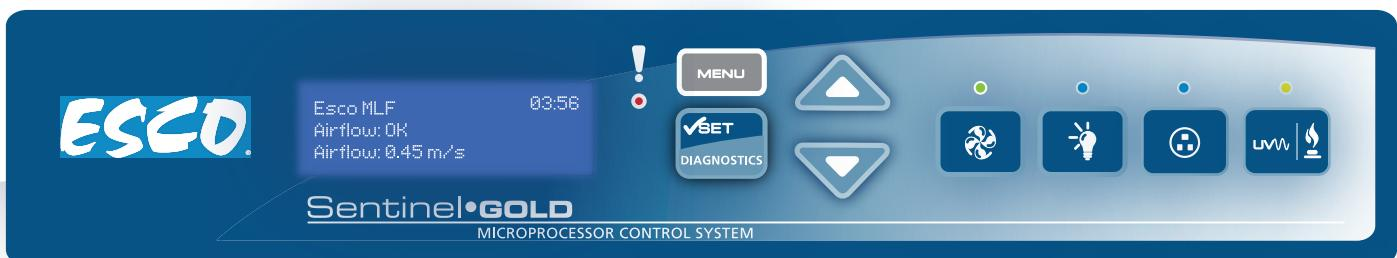
Displays all safety information on one screen; there's also the standby mode which allows users to switch to an energy saving mode when the cabinet is not in use.
